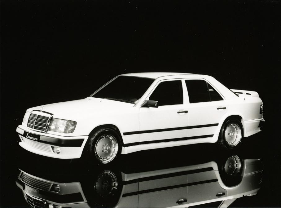
A Mercedes fresh from the body building salon: the wide-version 300E from Lorinser. The renowned South German tuner not only fits this grand limousine with its own bodywork parts and flared wheel arches in metal, but also provides its own sports chassis and Lorinser aluminium wheels. The complete bodywork conversion costs around 9,500 deutschmarks. Photo: Lorinser
